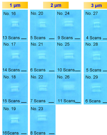
Figure 5 Microscope images of multi-line optical waveguides in LiTaO 3 crystals under perpendicular polarization. Left panel: trace intervals of 1 μm with 13-16 traces; middle panel: trace intervals of 2 μm with 5-11 traces; right panel: trace intervals of 3 μm with 4-6 traces. The white scale bar represents 30 μm.
